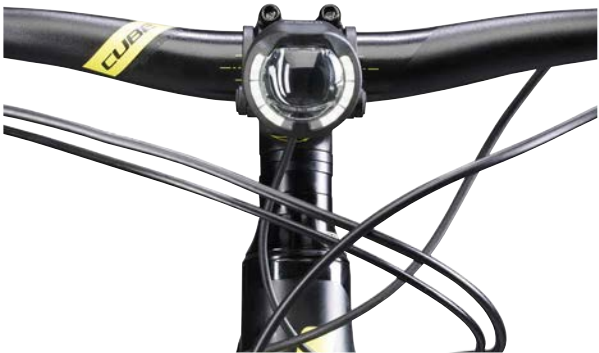
The SL detects the input voltage of 6 V or 12 V and automatically adjusts its performance.
